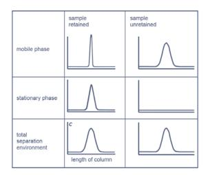
The diagram describes the chromatographic state of a non-eluted sample within the chromatographic bed (not to be mistaken for the concentration profile of an eluted peak). For an eluted peak the concentration of the sample within the eluent is plotted vs. the elution time or the eluted volume (c/t or c/R diagrams), and no longer includes considerations relative to the solid phase.
