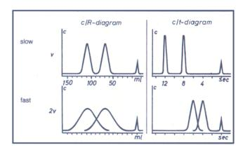
time within the sorbent bed. It is just as undesirable to "shoot" the sample through the bed because non-equilibrium of the solutes between stationary and mobile phases will also cause peak broadening.
