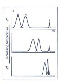
The point of saturation (S) is shifted to lower concentrations at higher temperatures. This temperature gradient exists with both adsorption and reversed phase systems. With rising temperatures the retention volumes for the various solutes decreases. Generally, the resolution and distance between the peak maxima (Äz) decreases, accordingly.
