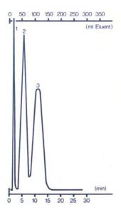
**4. "Dry-Column** Chromatography": This is a preparative chromatographic **technique** with resolution similar to thin-layer Chromatography<sup>171</sup> <sup>18</sup>> <sup>19</sup>
