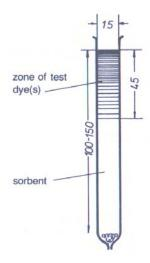
In the above example the sorbent shows a Brockmann activity of I/45. The test is performed using #1 solution, giving an activity grade I. The distance of migration is 45 mm, indicating the fine tuned position between activity grade I/O and I/50 for the production of the usual Brockmann grades I-V. One should choose deactivator to reach grade I/30, II/30, III/30 etc.
