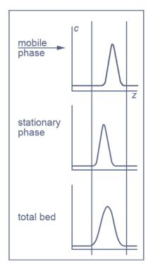
This phenomenon accounts for peak broadening due to mobile phase flow. It may be reduced but it can never be completely eliminated.
