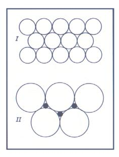
Similar reasoning also applies to irregularly shaped particles, especially when very small particles come close to the shape of a globe. The actual size (particle diameter) and the particle size distribution of an adsorbent play important roles in regulating column packing, pressure, and volume:
