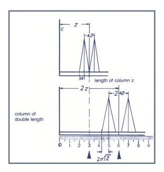
than necessary to achieve the desired separation. Excess column length leads to excess back pressure and an excess time of residence.
