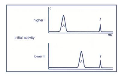
DAI adsorbents are standardized according to Brockmann and Schodder (see glossary). Due to this standardization, all chromatographic separations are absolutely reproducible over years when employing these products.
