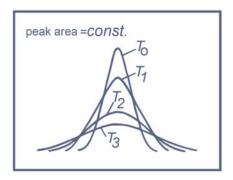
As a rule, (exemptions exist) the width at the base will continuously expand during the separation process. One of the prime tasks in chromatography is to apply the sample at a minimum width, i. e. with maximum concentration, while keeping the peak from broadening during the separation. As the initial peak becomes smaller, resolution is enhanced.
