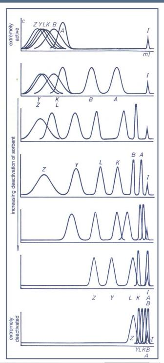
Despite identical initial activity, virtual standardization and the use of an identical mobile phase, chromatogram output may not always be the same. Only if both the initial activity and the deactivation behavior of an adsorbent are standardized to the highest degree will identical, reproducible and reliable separations be achieved.
