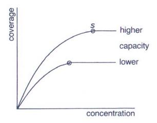
Sorbents having well defined and of highest possible activity – such as Alumina DAI Activity Super I and Silica DAI, Active - are preferentially used for purification purposes. Frontal analyses and bulk applications using agitated reactors are the main types of applications for high activity = high capacity sorbents.
