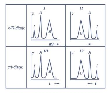
Graphic plots represent the time or volume axis and run on the paper from right to left or vice versa. If the paper leaves the recorder from left to right, plots are written from right to left, such as shown in graphs II and IV above.
