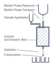
separated out is applied at the upper end using a pipette. The bulb acts as a reservoir for the mobile phase. The physical force of gravity forces the eluent down the sorbent bed. The migration of the constituents can be detected and the sample separated or fractionated with the aid of a number of glass beakers.
