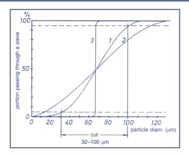
Standardized sorbents (curve 1) differ from non-standardized material (curve 2) in that the inclination of the sigmoidal curve is steeper with the standardized and in having only a low percentage of excess fines. They are also free from coarse particles which could impede homogeneous packing of the sorbent bed.
